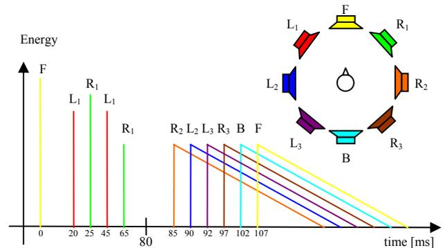
Image 1: Systematic drawing of the impulse response and the setup of the synthetic sound field.
