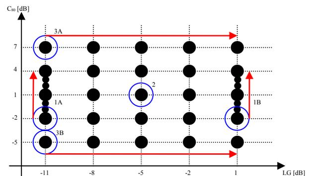
Image 2: Range of values covered in the listening tests. The blue circles mark the reference stimulus for the different experiments. The red arrows indicate the range of stimuli that were compared to the respective reference. Ref. 1A/1B: Exp. 1, Ref. 2: Exp. 2, Ref. 3A/3B: Exp. 3
